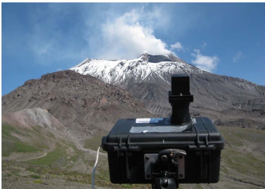
Figure 1.3: Photo of the FLYSPEC at Bezymianny Volcano. Measurements of absorbance of UV light by \text{SO}_2 in the volcanic plume at Bezymianny volcano are collected via horizontal above-vent scans. Photo taken July 2009.
