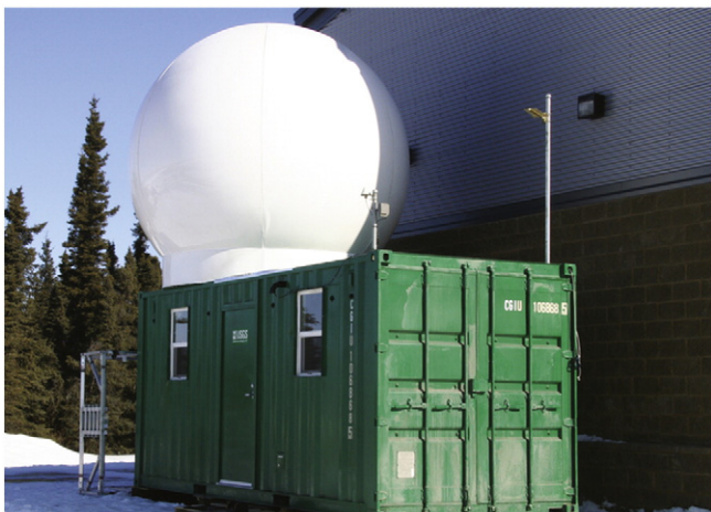
Fig. 1. MM-250C Doppler radar system deployed at the Kenai Municipal Airport.
