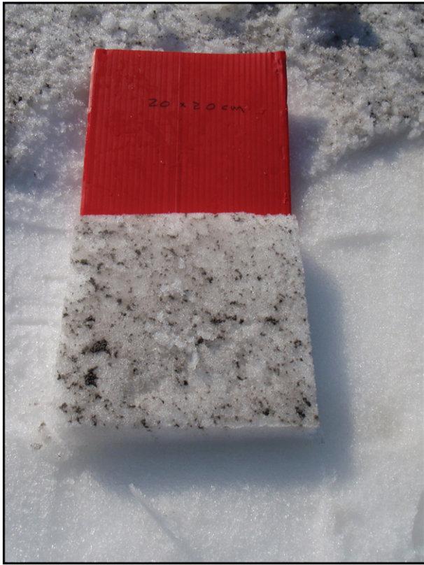
Fig. 3. Photograph showing an example of measured-area sampling guided by a 0.04 m 2 plastic template (red). Such samples yielded mass per unit volume measurements for contouring and calculation of total deposit mass (Fig. 1). Note the deposit thickness is ambiguous owing to compaction or melting of frozen aggregates pellets.
