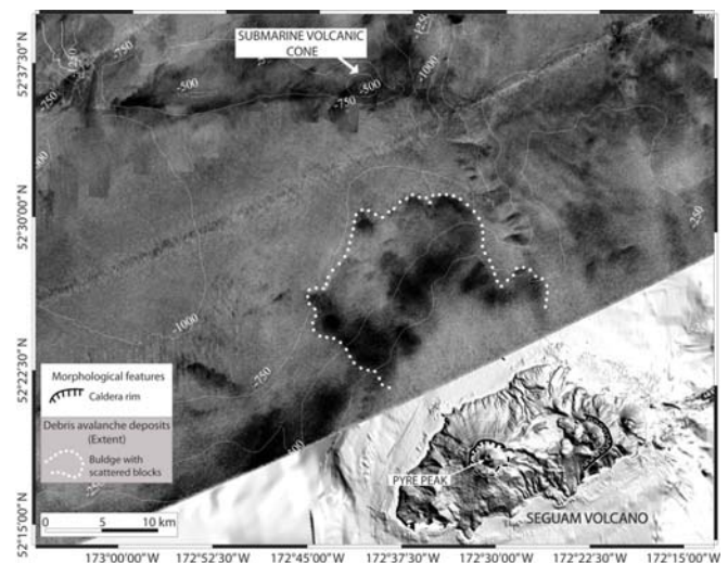
Fig. 11. Topography, bathymetry and Gloria side-scan data of Seguam Island and its northwest submarine part. On the north side a large submarine cone is also visible. For side scan data the black is high backscatter and white is low backscatter. Contour interval is 250 m.
