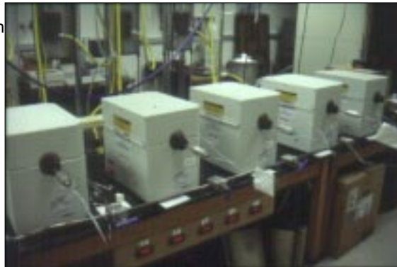
Figure 38: Photograph of the four new vertical furnaces. Note that a vertical pressure vessel with rapid quench extension is in place in one of the middle furnaces. Temperature controllers are grouped below the furnaces.
