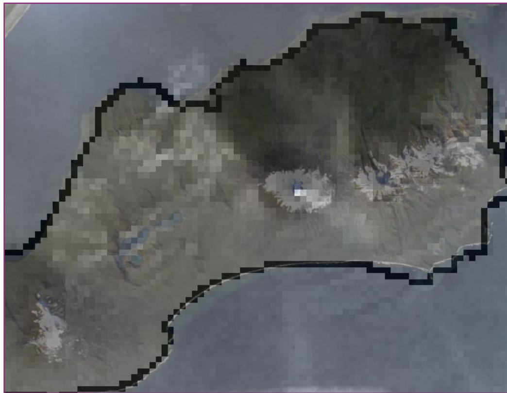
Figure 2. The thermal anomaly and steam plume in image n15.99040.1928 overlain on a space shuttle photograph of Unimak Island (STS047-077-034). Each AVHRR pixel is ca. 1.1 km on a side. The bright spot at the summit represents a temperature of 11 degrees centigrade. The zenith angle for this image was 14 degrees.
