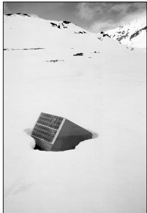
Figure 26: Station ISTK (South of Isanotski Volcano). Photo taken on 4 th July. Deep snow this last winter is probably the cause of the damage sustained by both solar panels.
