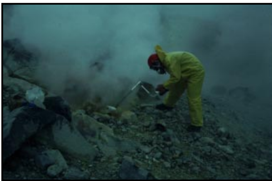
Figure 27: Photograph showing Bob Symonds sampling gases from the superheated fumarole on the south side of Mageik crater.
