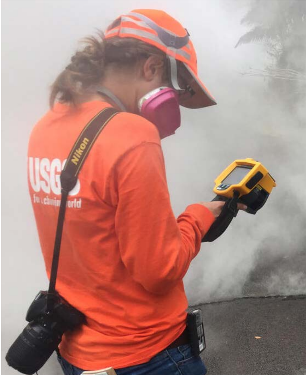
Photograph of Research Corporation of the University of Hawai'i scientist Liliana DeSmither measuring surface temperatures with a thermal imaging infrared camera from a road crack in the Leilani subdivision on the Island of Hawai'i during the 2018 eruption of Kilauea. U.S. Geological Survey photograph by Brian Shiro, May 9, 2018.
