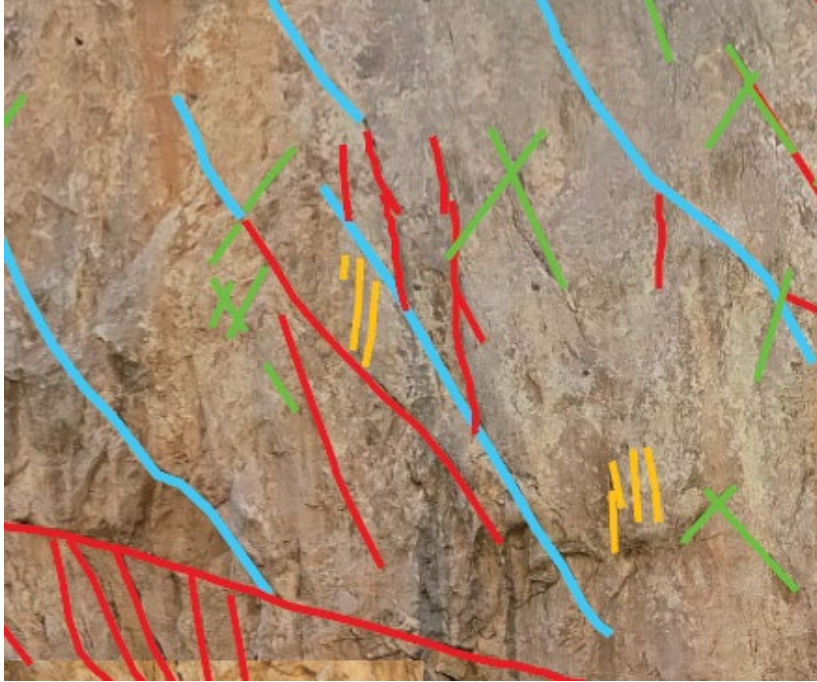
Figure 3.14. Faults (red) and bedding surfaces (blue) in places are difficult to distinguish. Without outcrop access bedding is mapped by its orientation and association with other bedding.
