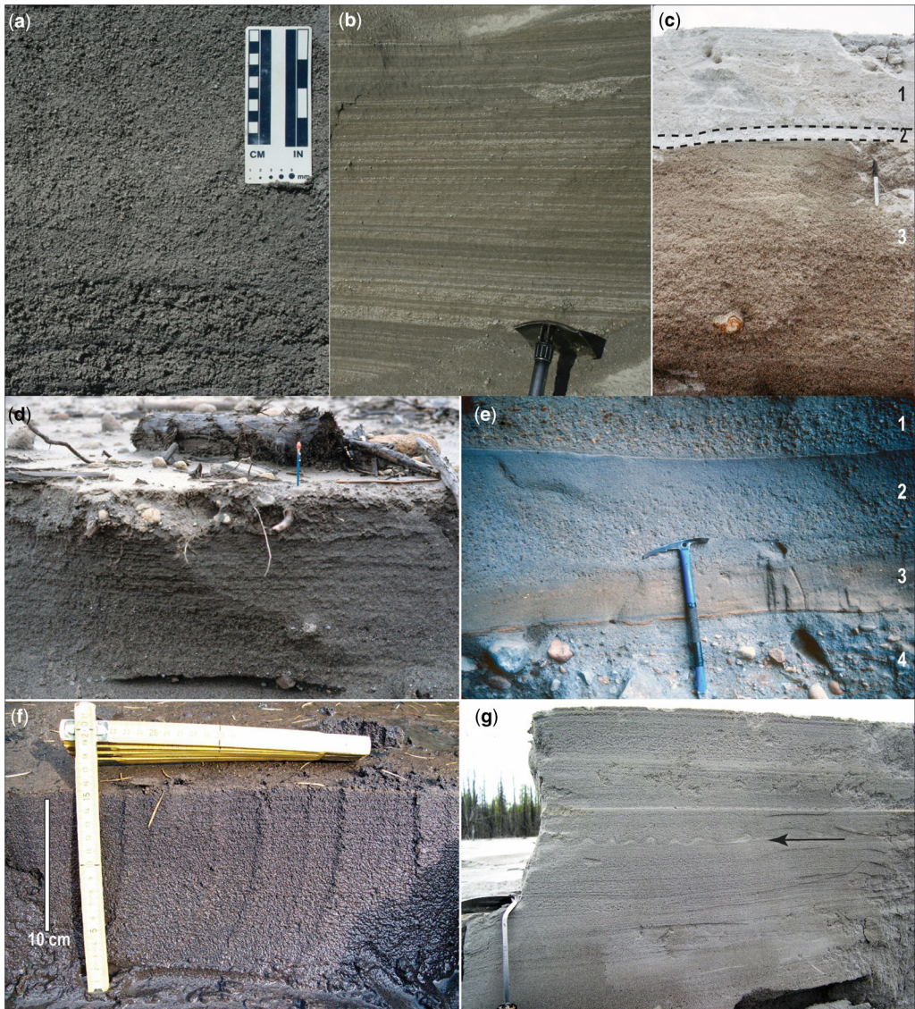
Fig. 26. Textures of type-2 (hyperconcentrated flow) lahar deposits. Note non-stratified to laminated textures, dominantly sand composition, and occasional coarse clasts. (a) Deposit from lahar that was relatively highly concentrated and near transition to type-1 lahar, Chaitén River, Chaitén volcano (Chile). Photograph by T. Pierson, USGS. (b) Horizontally bedded deposit from a dilute type-2 lahar, possibly verging on sediment-laden streamflow, Chaitén River, Chaitén volcano. Photograph by T. Pierson, USGS. (c) Non-stratified, normally graded type-2 lahar deposit (unit 3), underlying tephra fall (unit 2) and reworked tephra fall (unit 1), Abacan River, Mount Pinatubo (Philippines). Photograph by J. Major, USGS. (d) Deposit of non-stratified to indistinctly laminated coarse sand with entrained pumice particles within and atop deposit, Toutle River valley, Mount St Helens (USA). Photograph by T. Pierson, USGS. (e) Deposits from type-1 (unit 1) and type-2 (unit 3) lahars. The deposit juxtaposed with axe head (unit 2) represents a type-1 lahar in basal part and grades upward to sandy facies deposited by a type-2 lahar phase, Nisqually River valley, Mount Rainier (USA). Photograph by J. Major, USGS. (f) Non-volcanic hyperconcentrated-flow deposit emplaced by flow having a sediment concentration of about 26% by volume, White Salmon River (Washington, USA). This deposit resulted from flow shown in Figure 19d, a flow generated by a dam removal. Photograph by J. O'Connor, USGS. (g) Stratified fine to medium sand deposited by a type-2 lahar from April 2009 eruption of Redoubt volcano (USA). Convoluted bedding (arrow) indicates rapid loading of water-saturated sediment. Photograph by T. Pierson, USGS.
