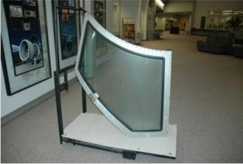
Abraded windscreen from the Boeing 747 damaged in the December 15, 1989 eruption of Redoubt Volcano. The frosted right side of the glass almost completely obscured the pilots ability to see out; on the left, the clearer, less-abraded side received only glancing blows from ash particles as the plane flew through the ash cloud. This instructive piece of aviation history is housed at the University of Alaska Anchorage in Anchorage.
