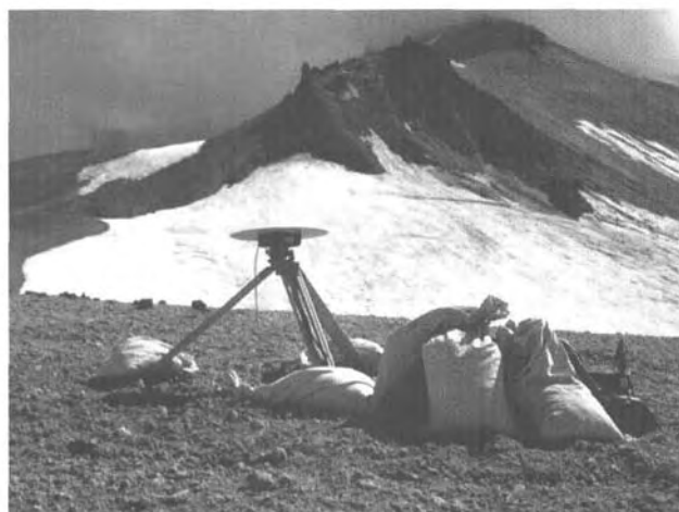
Figure 2. The Mainstreet GPS station located on the northwest slope of Trident Mountain. The GPS receiver and battery are located under a plastic tarpaulin weighted down by tephra filled sample bags in the left foreground.
