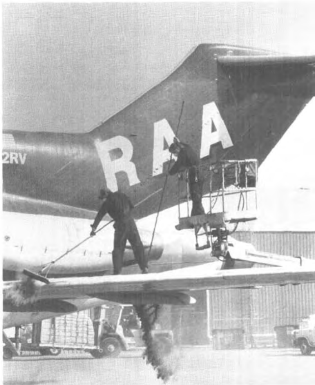
Figure 3. Maintenance crew removing ash from wing of a Reeve Aleutian Airways Boeing 727-100 aircraft on August 19, 1992, at Anchorage International Airport. Photograph by Erik Hill courtesy of Anchorage Daily News.
