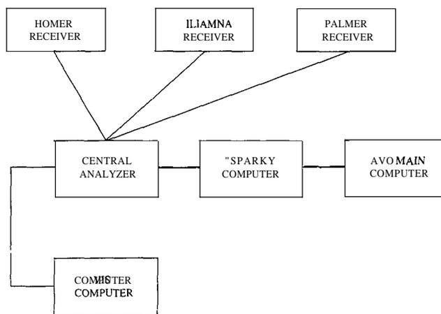
**Figure 2.** Data storage and communication links for Alaska Volcano Observatory's (AVO) lightning detection system. The central analyzer queries (via modem and phone line) each remote receiver at user-defined intervals. Incoming data are stored in the central analyzer and the computer named "Sparky." Data can be manipulated and viewed graphically through the video information system (VIS) and the AVO main computer.
