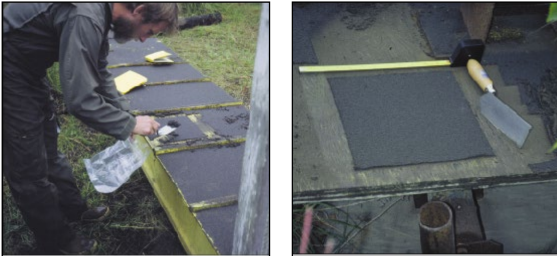
Figure 2. Collection of measured-area tephra samples from hard surfaces after 1992 eruption of Crater Peak/Mount Spurr, AK (photo from September 21, 1992).
