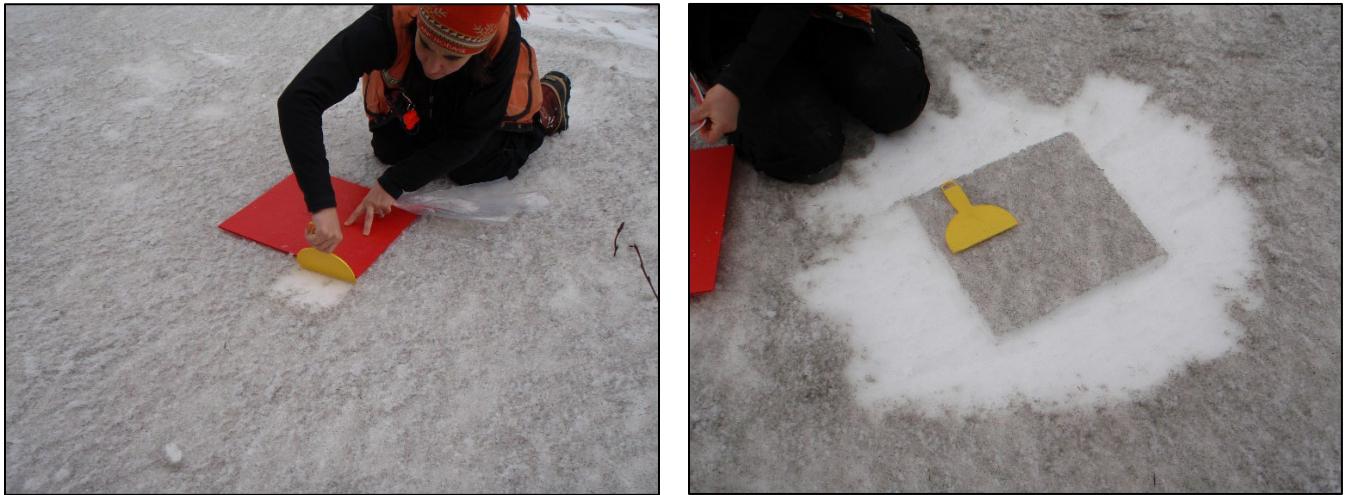
Figure 1. Collection of measured-area ash samples from snowpack after the 2009 eruption of Redoubt volcano, AK (photo taken on March 7, 2009).
